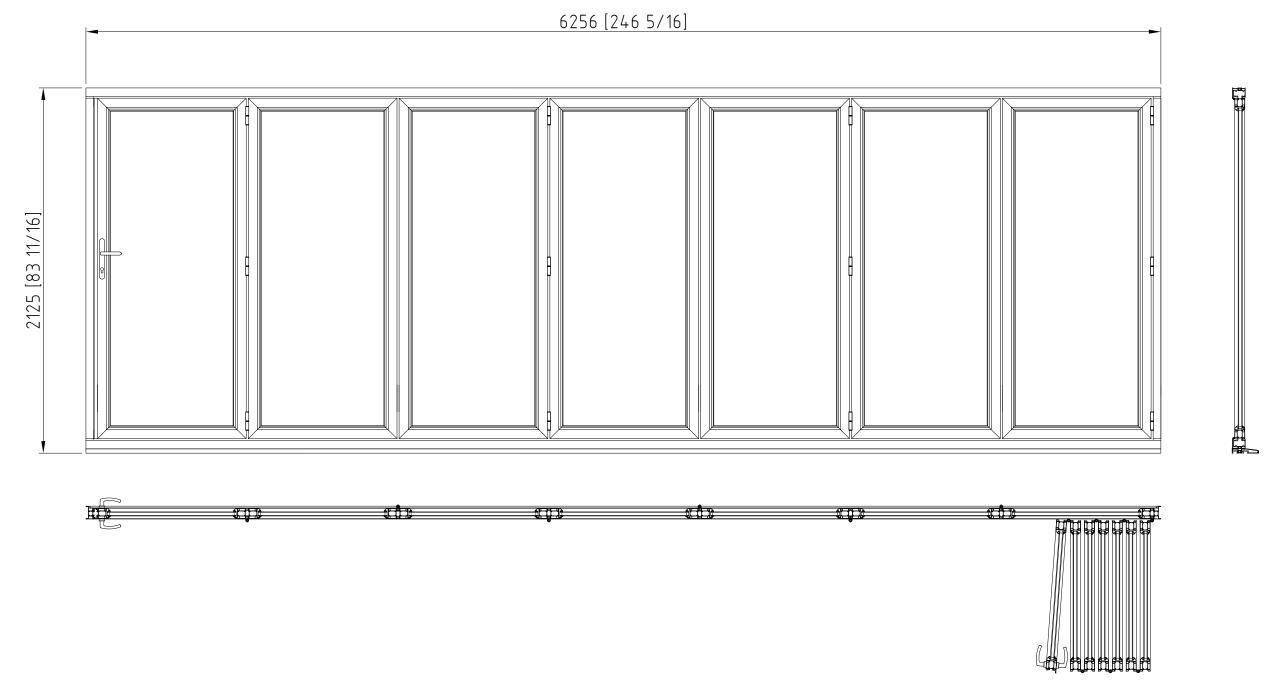
Suitable for apertures 2800mm [110 1/4] to 8400mm [330 3/4] wide and upto 2500mm [98 3/8] tall
