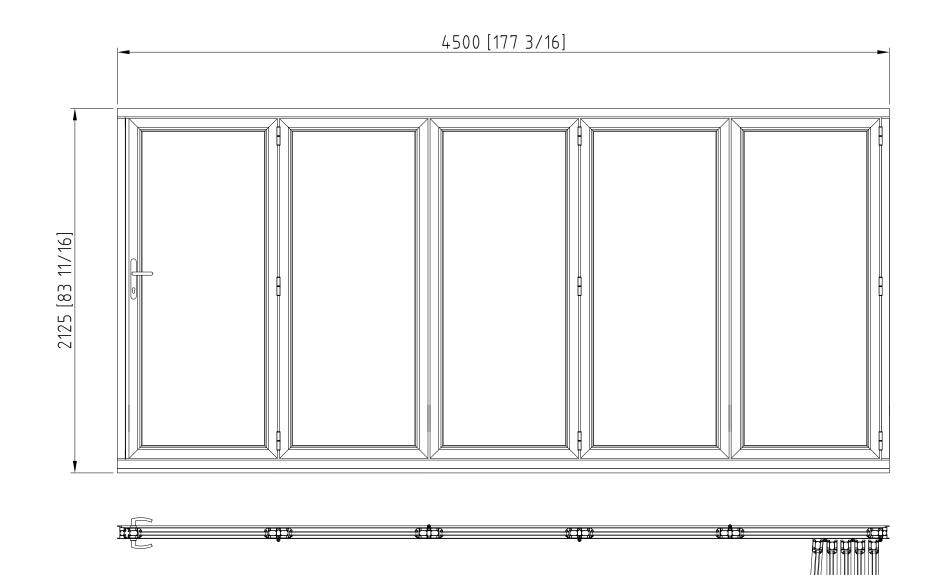
Suitable for apertures 2000mm [78 3/4] to 6000mm [236 1/4] wide and upto 2500mm [98 3/8] tall
